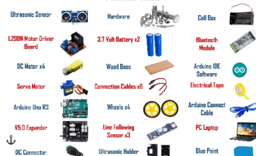
Figure 2: Diagram of materials used to construct the robotic vehicle
