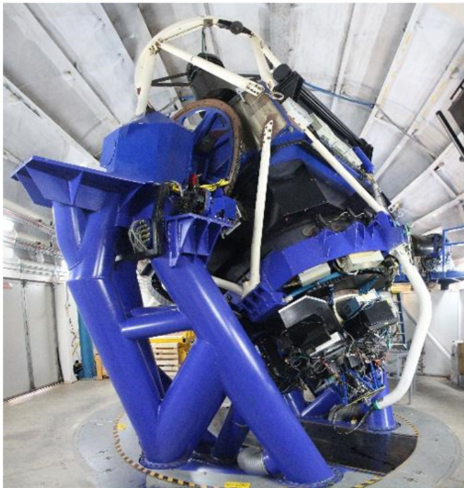
Figure 2: Highest Aperture (2 m) Robotic Telescope Used (Faulkes Telescope South) Image Credit: Gronk Oz - Own work
