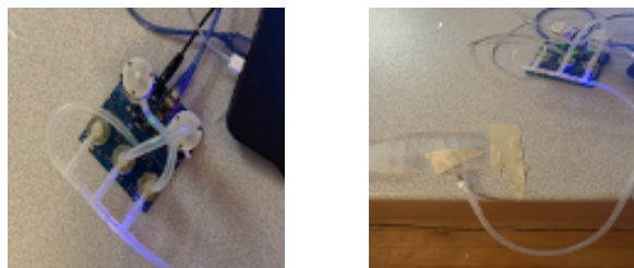
Figure A1: Programmable Air with connection to computer with Arduino software and connection to pneumatic pouch motor.
