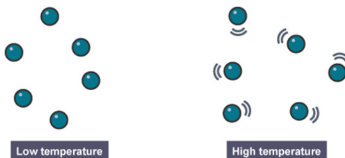
Figure 5. Diagram of how particles move slower in low temperatures compared to the particles at high temperatures [5].
