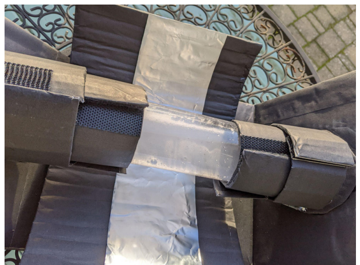
Figure 1: SODIS Water Bottle Holder Device Under the Sun. Prototype of the SODIS device that has aluminum foil in a parabolic shape to reflect UV rays onto the water. A plastic water bottle was placed and secured into the SODIS device at a flat 180-degree angle.
