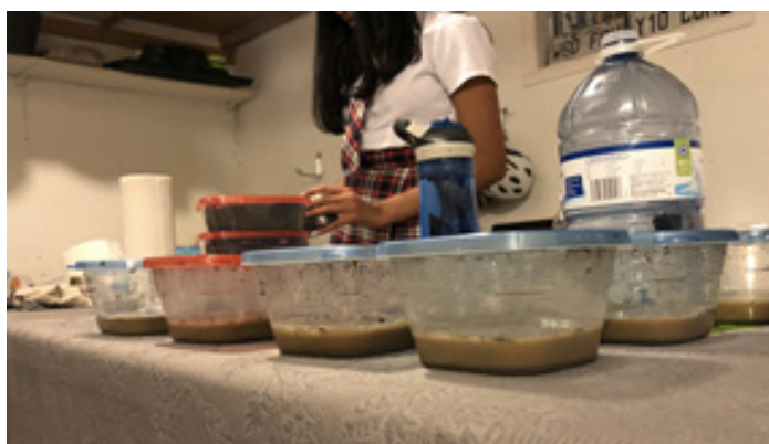
Figure 2 Separation of the Soil from the Desired Solution. The separation process lasted between a few hours and a few days depending on the texture of the soil (clay soils required more time than sandy soils).
