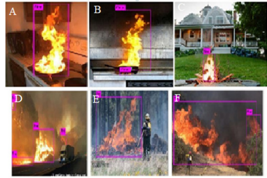
Figure 7: Images A, B and C show detections made on the single flame dataset. Images D, E and F show detections made on the high-risk fire emergency dataset. These detections demonstrate the model's ability to perform in many different settings and conditions.
