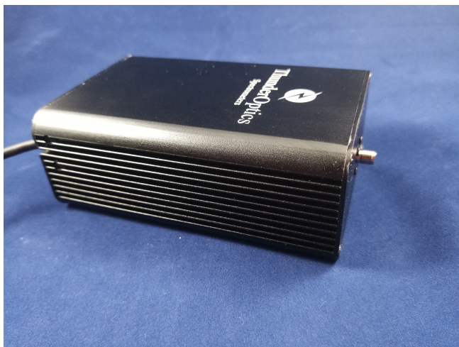
Figure 3. Optical Spectrometer used for measurement of intensity of light at different wavelengths, i.e. a spectrum.
