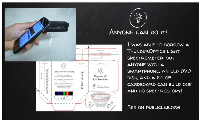
Figure 8. Foldable cardboard spectrometer [3] can be built with a smartphone camera, a piece of an old DVD, and some cardboard.
