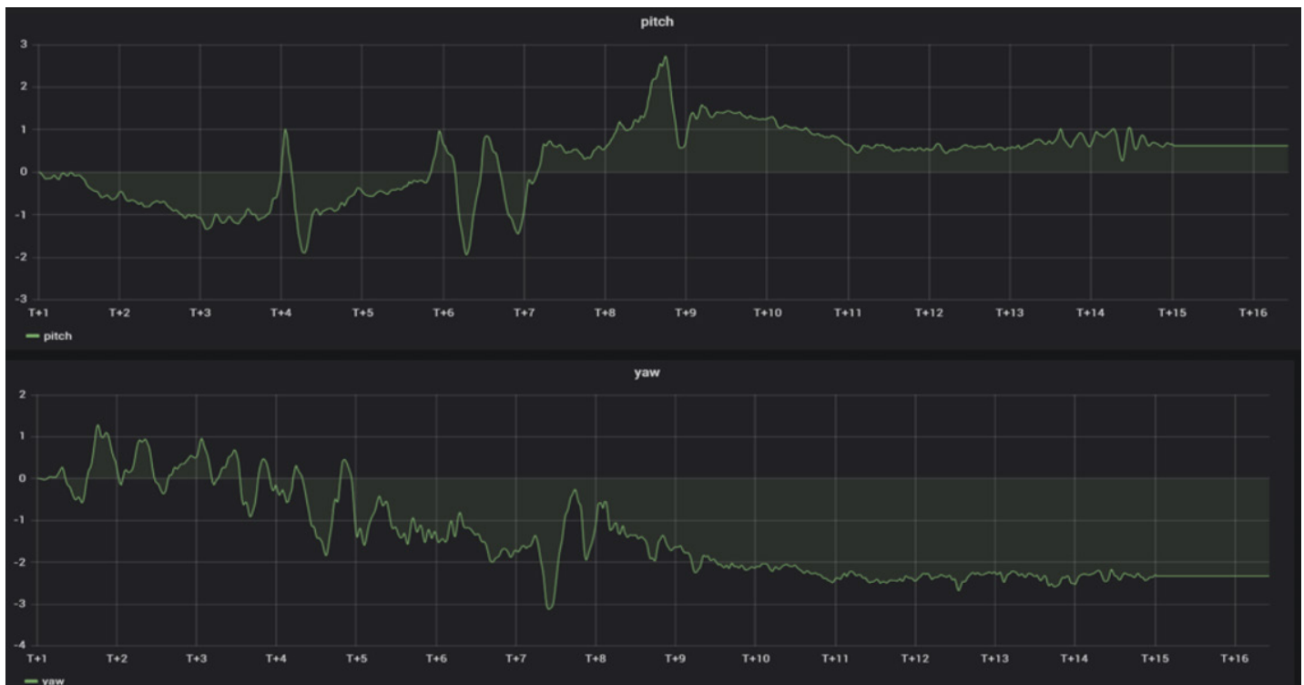
Figure 6: Data from a Revision 2 ground test x axis is time on both graphs. Upper graph is pitch; lower graph 2 is yaw.
