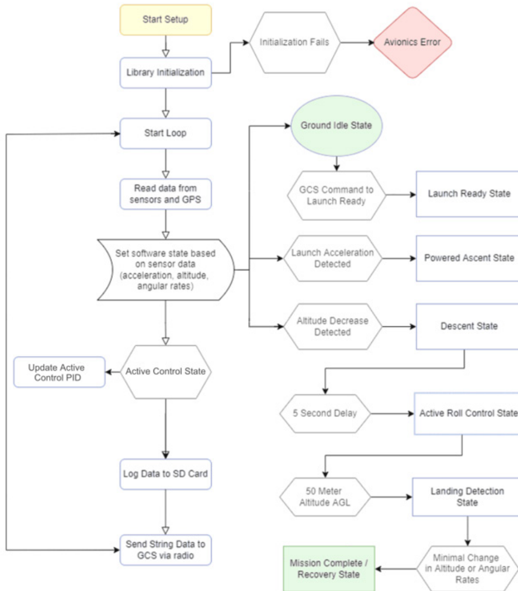
Figure 3: A flowchart of different software states of the test vehicle
